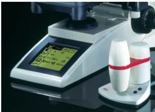
Left: The new LeicaScreen on the DM6000B with touch-sensitive LCD display. The clearly designed menu structure uses internationally familiar pictograms* instead of language for intuitive operation. Right: The familiar Leica SmartMove remote control. You can use the remote control unit to control all 3 axes of the microscope (x,y: stage, z: focus). You can also program user-defined microscope functions and assign them to the 4 function buttons.
