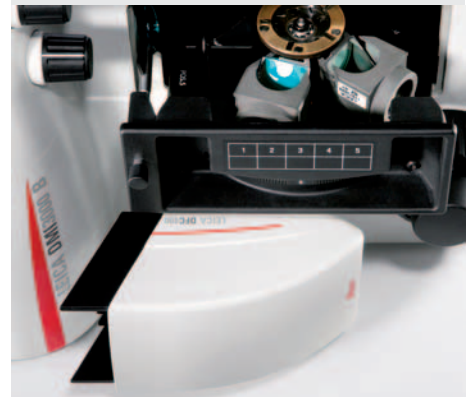
5-position manual fluorescence turret
