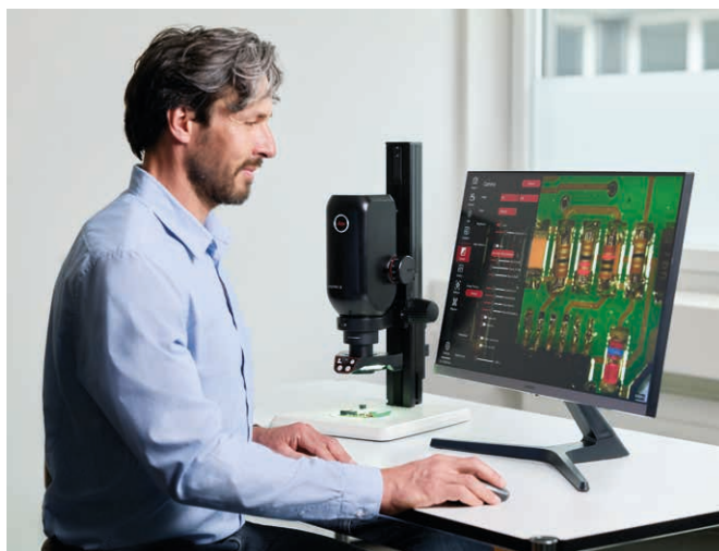
Emspira 3 digital microscope with standard base and LED3000 ring light illumination.
