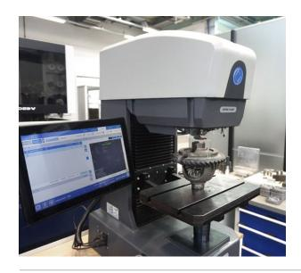
The Wilson\* UH4000 series universal hardness tester is designed for high volume production labs and production floors. The UH4000 series is available in two load configurations, UH4250 and UH4750. Universal testers are designed to be capable of performing several hardness scales; in most cases, testing with higher loads (>5kgf).
