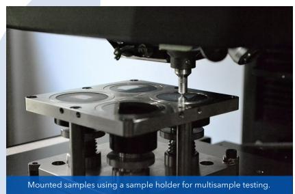
The motorized stage can be used to perform also microhardness testing, e.g. CHD testing using loads from 0.5kgf. Our standard sample holders for mounted samples fit on the stage and are secured with magnets.
