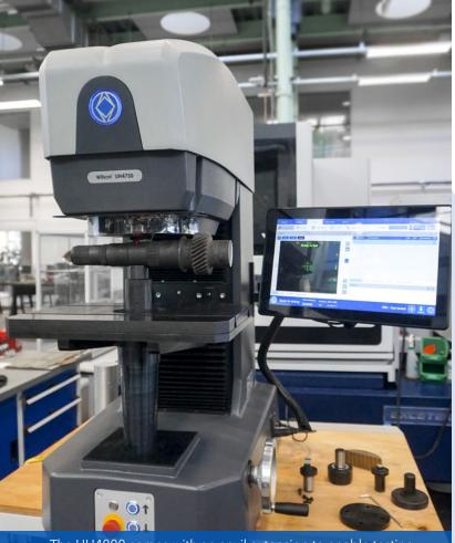
The UH4000 comes with an anvil extension to enable testing of smaller or cylindrical parts.
