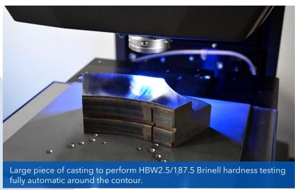
Bigger parts, such as castings, or sectioned pieces of castings and forgings can be easily placed on the stage to perform full automatic Brinell testing. Loads are applicable up to 250kgf, test piece weight up to 50kg.
