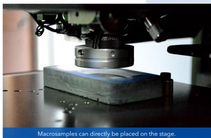
Large crosssections of welds or other type of materials can be easily placed on the motorized stage and automatically tested. The macro objective provide scanning capability to achieve a complete overview image of the sample.
