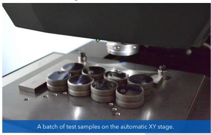
Batch testing is carried out when a large quanity of samples need to be verified. Testing is usually done on the complete part itself or on representative pieces of the complete part. Different test methods can be used, Rockwell testing is the most common one for heat treated parts. DiaMet can program the same or different test patterns per piece and fulfil a complete automatic test sequence, i.e. automatic test pattern placement and measurement.
