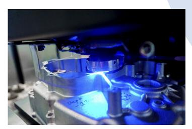
The Wilson UH4750 and UH4250 work perfectly for all kind of casted components, like engine and transmission cases. Brinell testing is carried out with HBW2.5/62.5 or HBW5/250 test scales, when using Al based castings, and HBW2.5/187.5 or HBW5/750 test scales, when using Fe based castings.
