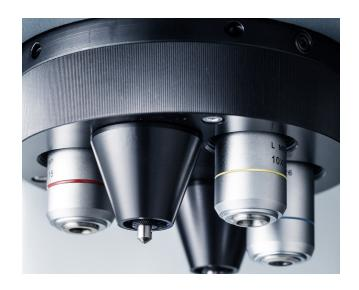
The precision mechanics of the motorized turret, allow for a fast and quiet positioning. Switching between indenter and objective is part of the automated test cycle.
