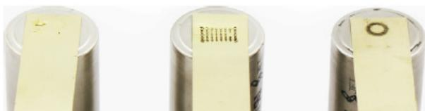
Figure 9 illustrates the common welding techniques of lithium ion batteries with left - spot weld, middle - ultrasonic weld and right - laser beam welds interconnects on Li-Ion cylindrical cells, (Martin J. Brand, 2015).
