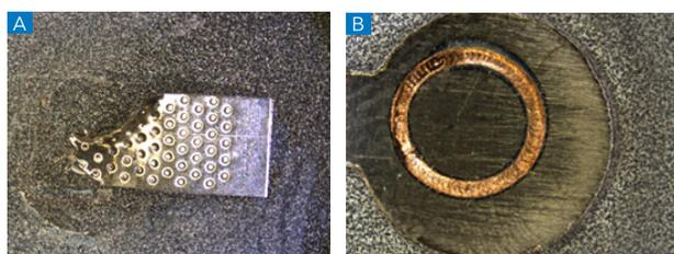
Figure 10 shows examples of (a) ultrasonic and (B) laser beam welds before cross-sectioning and castable mounting to investigate the quality of the weld.
