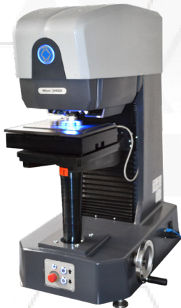
UH4250 Universal Hardness tester, 0.5 to 250 kgf, Rockwell regular & superficial, Vickers, Knoop, & Brinell testing
