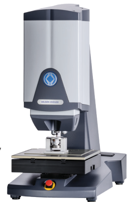
VH3300 Vickers-Knoop Automated Hardness tester, 0.01 to 50 kgf, ASTM E92, E384, E10, ISO 6507, 4545, 6506
