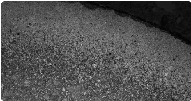
Structure of steel which has undergone decarburization. The sample is from an electric motor shaft.
