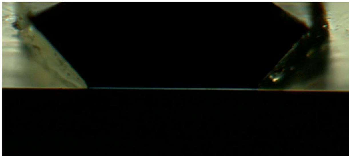
Using this method, an alignment with a deviation of less than 1  $\mu\text{m}$  is possible over the entire block face. A blue light gap, where blue light is reflected from the block face typically indicates a distance of approximately 400 nm between the block face and the knife. An evenly distributed light gap across all angles at this distance is the most precise indicator of a correct light gap setting, which ensures minimal loss of material. The solution
