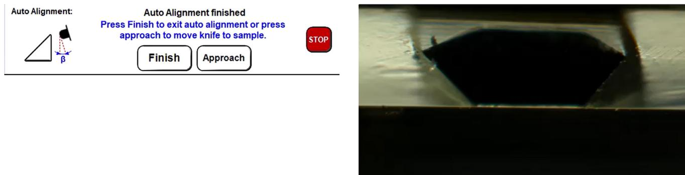
Figure 12: Final approach to the sample with safety distance of about 5  $\mu\text{m}$ . Left: The user can decide to approach the sample automatically or manually after alignment. Right: Light gap after approach. A safety distance of about 5  $\mu\text{m}$  will be kept.
