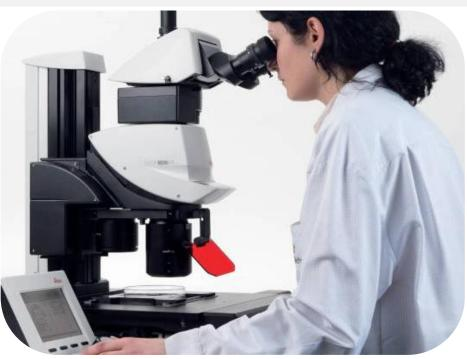
4. Close your left eye and adjust the right eyepiece (focus) until the image is sharp. Now repeat this process with the left eye. If the microscope only has one adjustment, you only need to adjust one side.
