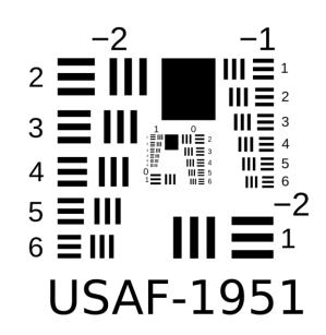
Resolution test charts have been used since the late 19th century to evaluate and calibrate the resolving power of imaging systems such as microscopes, cameras, and optical devices.
