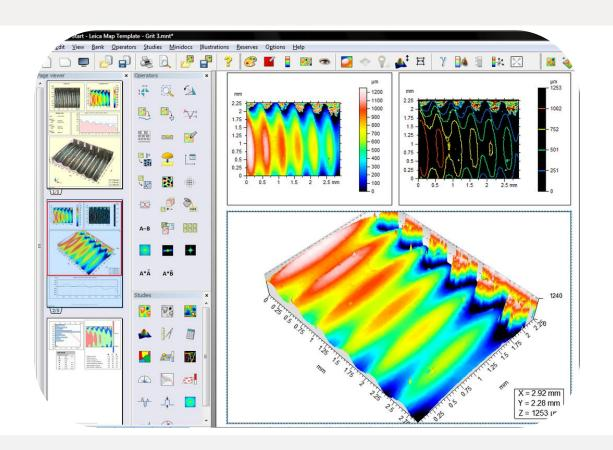
**Leica Map** is used for viewing and analyzing surface geometry and surface texture from LASX depth map images.
