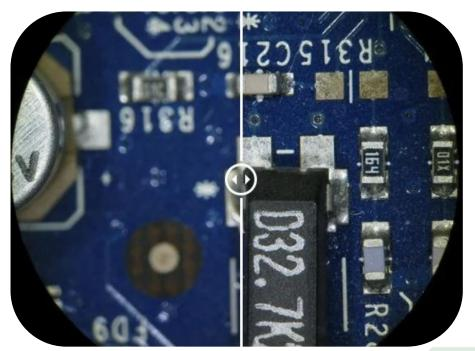
**5.** Check parfocality by going back to the highest magnification and focusing on a sample. Do not re-adjust eyepieces or tubes. Now go to the lowest magnification. The sample should stay in focus.
