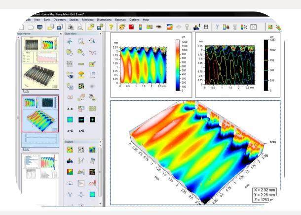
**Leica Map** is used for viewing and analyzing surface geometry and surface texture from LASX depth map images.
