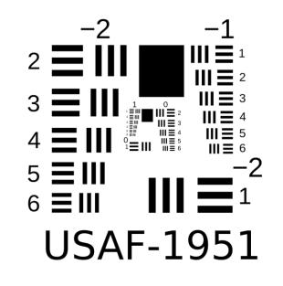
Resolution test charts have been used since the late 19th century to evaluate and calibrate the resolving power of imaging systems such as microscopes, cameras, and optical devices.
