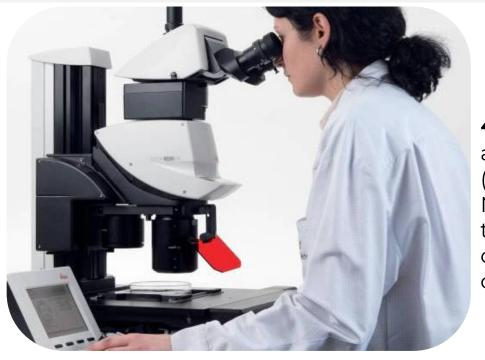
**4.** Close your left eye and adjust the right eyepiece (focus) until the image is sharp. Now repeat this process with the left eye. If the microscope only has one adjustment, you only need to adjust one side.
