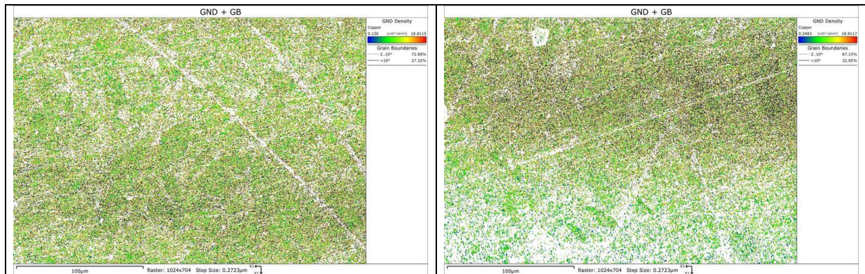
Figure 2. GND density after Mirror Polish (left: as-received, right: annealed). Both maps are showing elevated values across the whole field. The prep damage layer is dominating everything.
