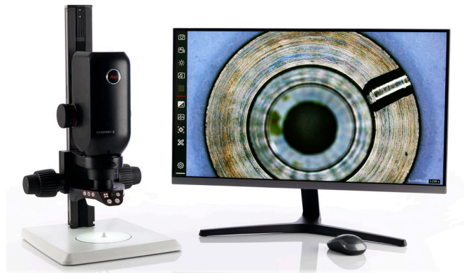
Emspira 3 digital microscope operated with the on-screen display (OSD) of the Enersight software platform.
