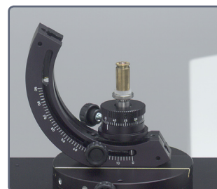
Push-in mounts available for caliber 0.22 – 0.45
