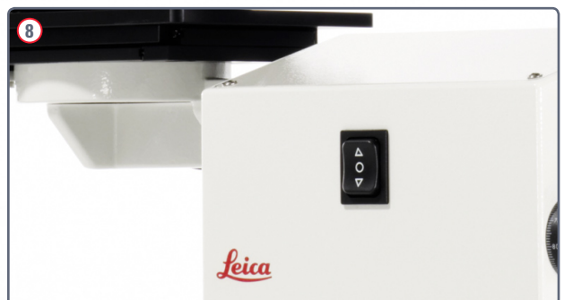
A unique feature of the FS M is the synchronized movement of both stages in x direction.
